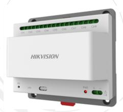
DS-KAD709 is the integrated equipment for supplying power to two-wire indoor station and door station. Its two-wire interfaces and adaptive network interface can support 9 devices and one external switch respectively. Its ingenious design enables it to be mounted on the DIN rail.
