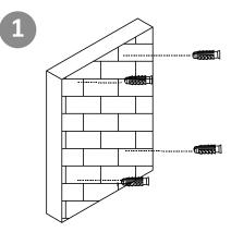
Insert 4 expansion tubes into the wall.
