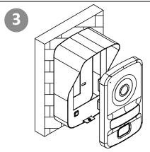
Install the door station into the protective shield. Distributed by
