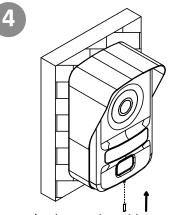
Secure the door station with a set screw.
